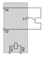
**NOTE:** For DC input, A1 have to be +, otherwise it would short circuit from protection module
